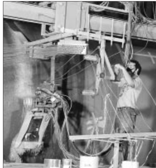
Structural wall is constructed by simultaneous glass chopping, resin spraying and hoop filament winding. (Winding glass is visible at top of photo.)
