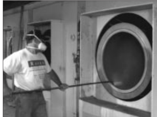
Each layer of glass and resin is rolled to remove air bubbles and to insure a dense uniform laminate.
